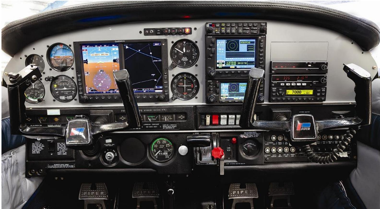
Piper PA28 with Garmin G600 EFIS and dual GNS-W.
