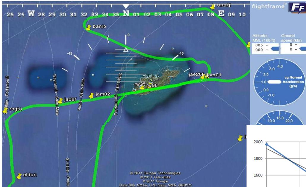
Data recorded using a Shadin Avionics portable GPS logger and data imported into Google Earth for map overlay.
